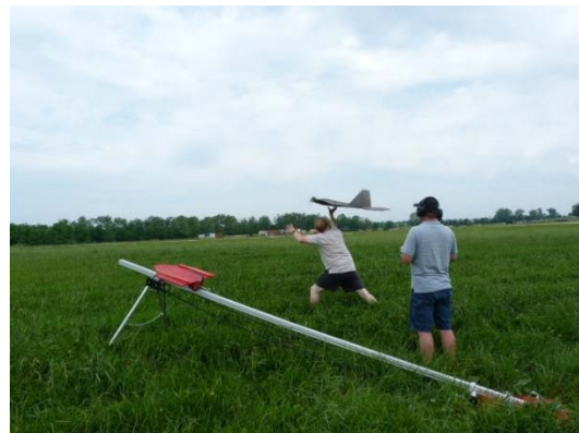
Fig. 9. Launch catapult and hand launch.
